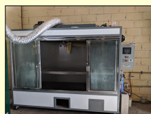
Figure 2. A bench type track sprayer used for mesotrione application
