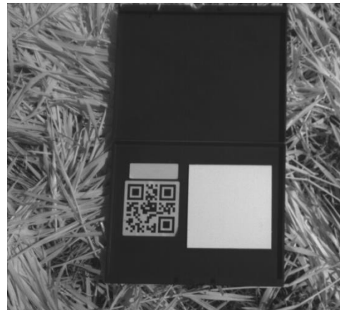
Figure 2-11. MicaSense RedEdge calibration reflectance panel. Photograph credit: Antonio Ray Asebedo.
