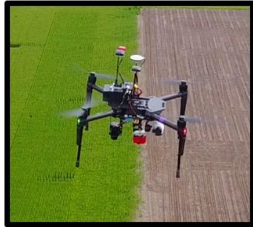
Figure 2-10. DJI Matrice 100 Platform Equipped with DJI X3 and MicaSense RedEdge. Photograph credit: Antonio Ray Asebedo.
