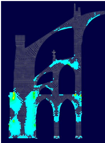
Figure 9.1 – Tensile Stress Distribution of Notre-Dame de Paris
