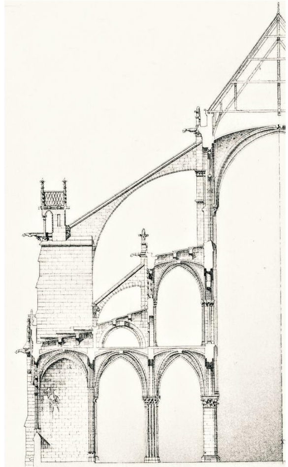
Figure 7.4 – Cross Section of Notre-Dame de Paris
