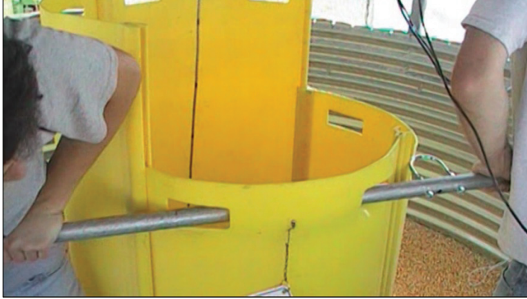
Figure 3. Grain rescue tube panels being manually inserted into the grain mass with a pipe running through the panel's hand-holds.
