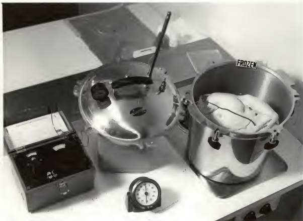
Fig. 2. Thermocouple and L & N Potentiometer Indicator arrangement used in pressure cooking.
