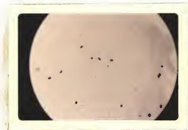
Figure 6. Coacervate droplets formed in 50 ml. of 1% starch paste by the addition of 2 grams of chloral hydrate in 50 ml. aqueous solution at pH 6.5. Stained by I_2KI . Magnification 475X.
