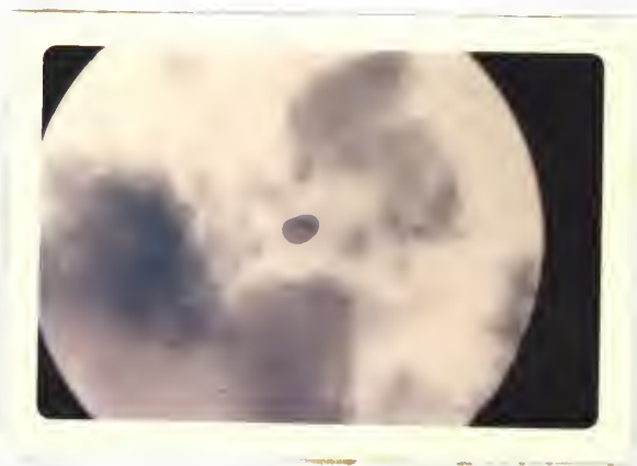
Figure 11. Coacervate droplet formed upon evaporation of a 1% starch paste. Stained by \text{I}_2\text{KI} . Magnification 475X.
