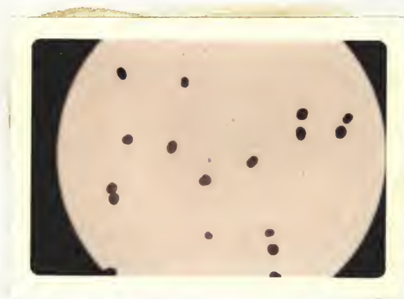
Figure 7. Coacervate droplets formed in 50 ml. of 1% starch paste by the addition of 8 grams of chloral hydrate in 50 ml. aqueous solution at pH 6.5. Stained by I_2KI . Magnification 475X.
