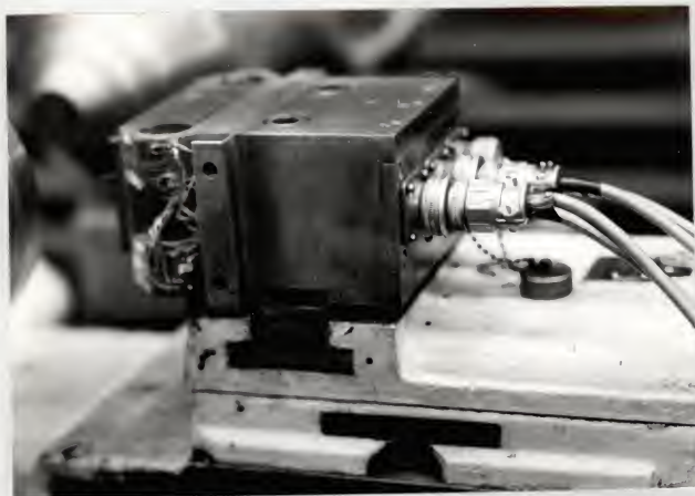
Fig. 6(b). View of the dynamometer exposing the strain gages.
