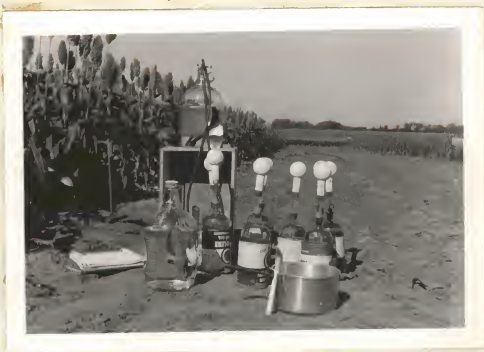
Fig. 3. Method and equipment used to clean atmometers between series.
