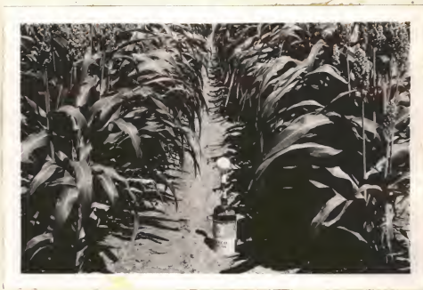
Fig. 1. Atmometer in 40" row width, showing method of placing and location in row.
