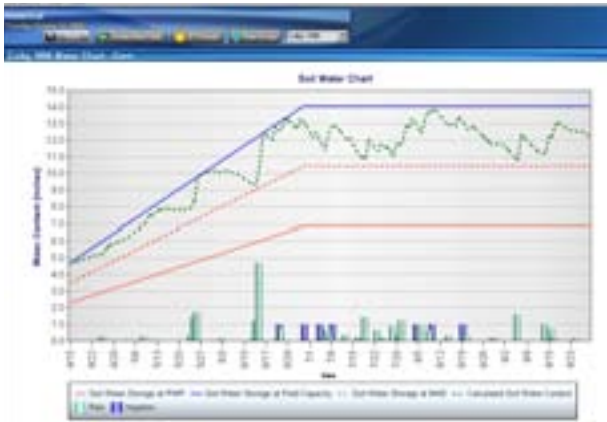
Figure 10. The Soil Water Chart section of KanSched2.
