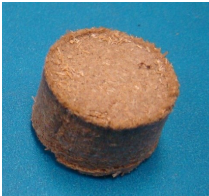
Figure 6-4 Picture of a pellet produced by UV-A pelleting
