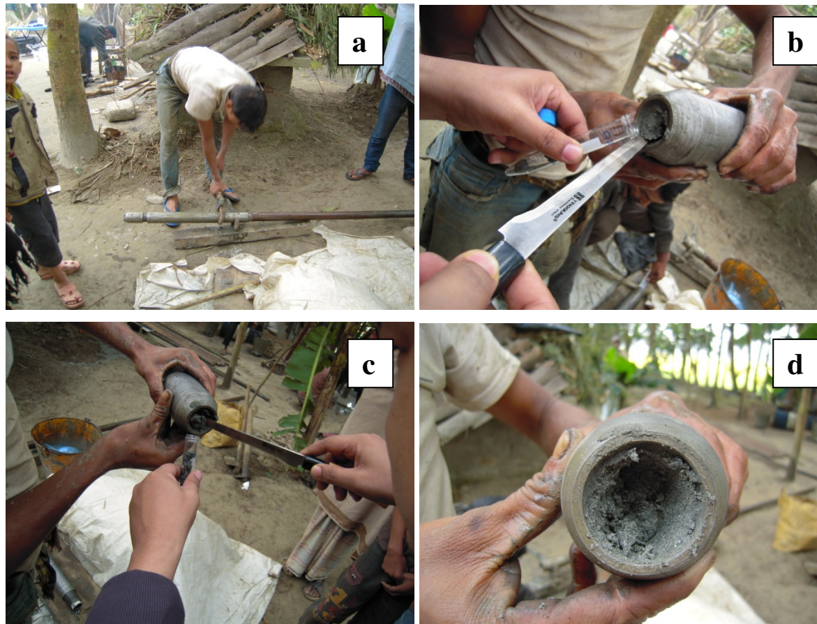
Figure 4.7 Microbial sediment sample collection method in the field after recovery of a core; a) separating the split spoon sampler from drill pipe; b) & c) taking fresh sediment samples for microbial testing in a sterile BD centrifuge tube; d) sample liner before separating from split spoon sampler.
