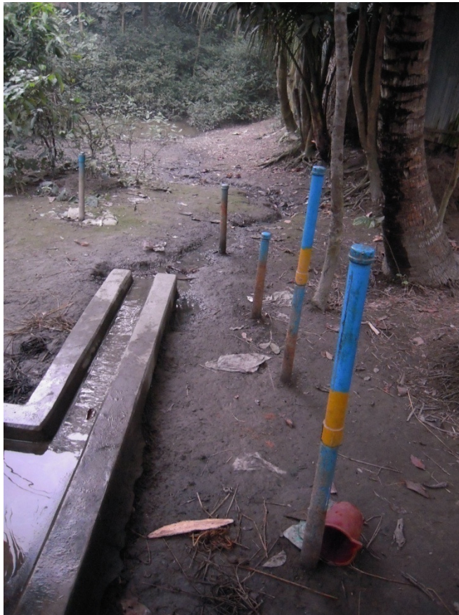
Figure 2.3 Piezometer Nest in North Matlab (Nest- 9)
