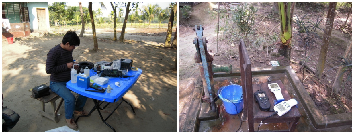
Figure 4.8 Testing for different field parameters using test kits after setting up a small working lab in the field site
