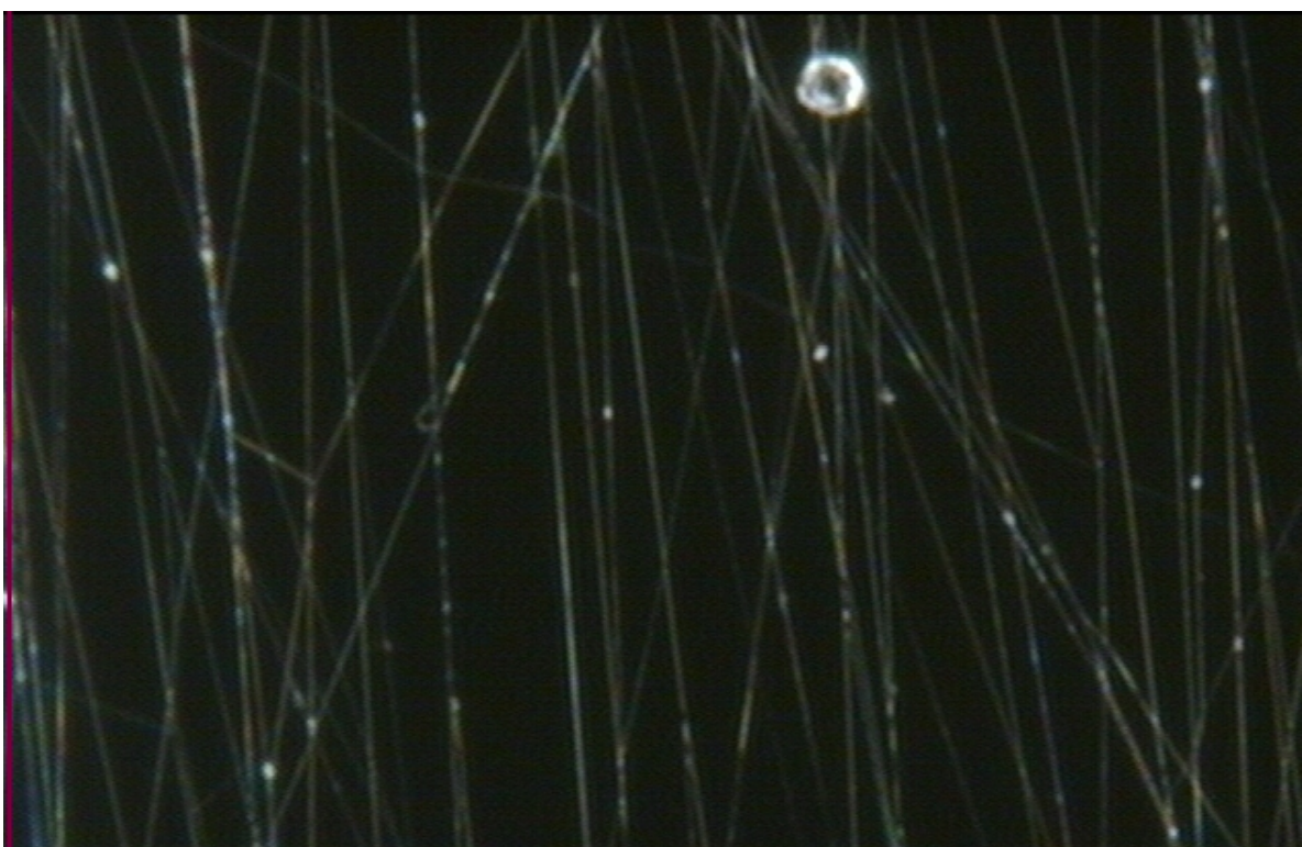
Fig 5.6: Aligned Fibers when vacuum was not used
