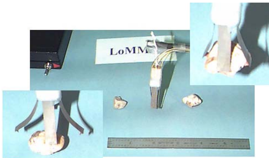
Fig 2.11: An end-effector gripper lifting 10.3g rock using four 0.1g fingers made of IPMC's. (Source: Shahinpoor et al. 1998)
