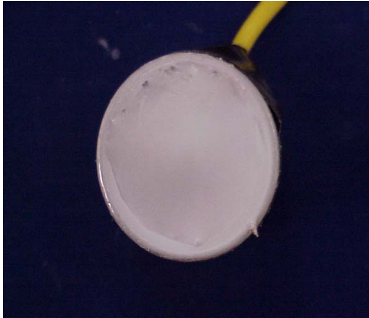
Fig 4.3: Images of the deposited nanofibers collected on a Circular shaped collector
