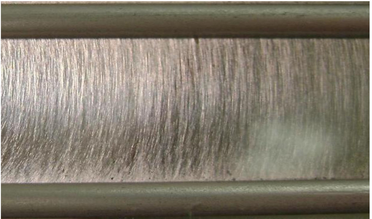
Fig 5.4: Fibers deposited parallel between electrodes
