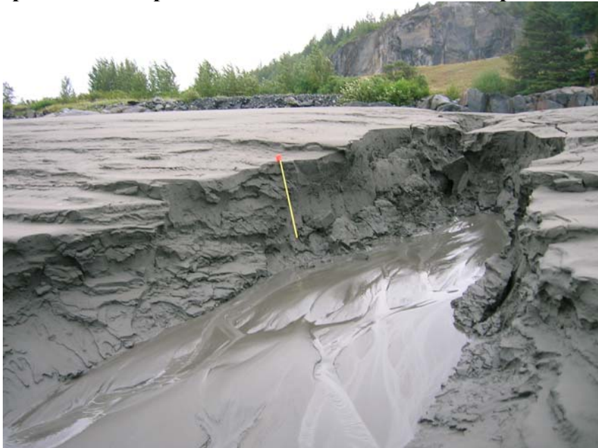
Figure 4-8: Large gully at EBP. Run off from the surrounding area was concentrated by a small ditch which emptied onto this portion of the bar. Scale at center of photo is 1 m.
