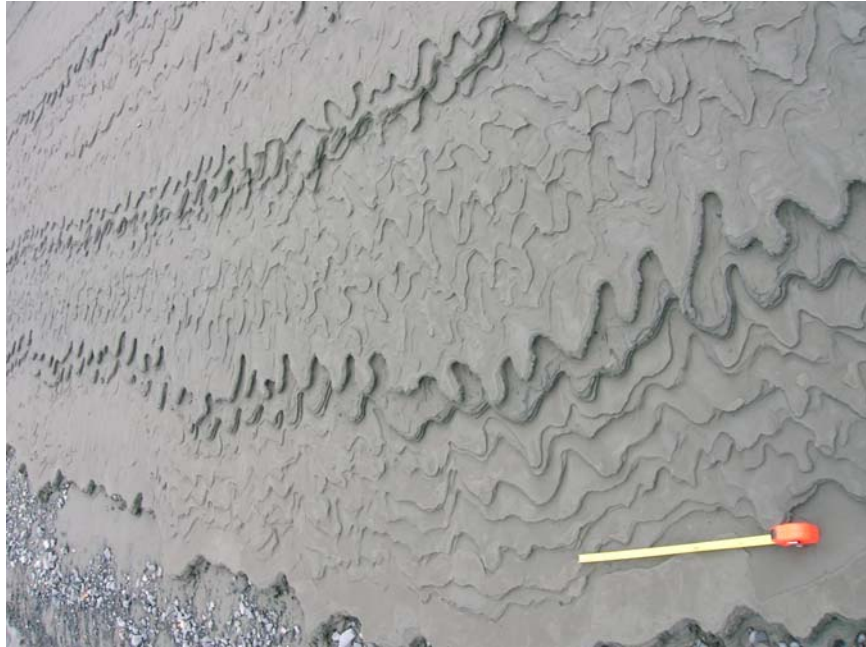
Figure D-3: Erosion of rippled surfaces. Scale is 50 cm.
