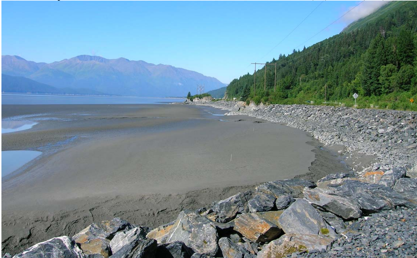
Figure 5-23: TBO4 on August 8, 2007, after high tide #23. Flats have developed to the west and the main channel has shifted south. Rods 2-2 (far) and 2-3 (near) are visible.
