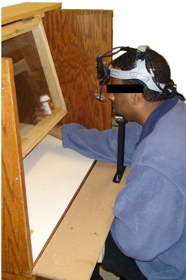
Figure 5. Experimental set up (chin rest, calibrated plane and the head-mounted optics of our ASL 501 eye tracking unit). doi:10.1371/journal.pone.0038819.g005
