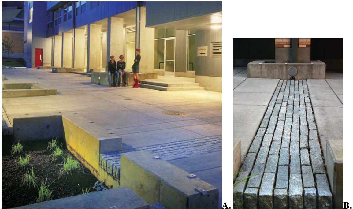
Figure 2.9 A: Picture of rainwater plaza. B. granite runnel and rock basin detail—Stephen Epler Hall, Portland State Univ.
