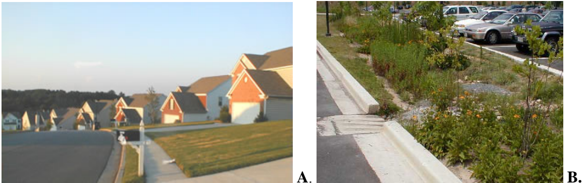
Figure 3.6 A: Connected impervious areas, and B: Disconnected impervious areas (Source: EPA, 2008)
