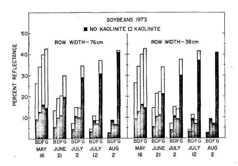
Fig. 4. Spectral reflectance for soybeans planted May 14, 1973. May 16 data taken on uncultivated soil without vegetation. Sensors B, D, F, and G measured spectral bands centered at 450, 545, 655, and 750 nm, respectively.
