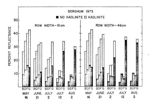
Fig. 2. Spectral reflectance for sorghum planted June 1, 1973. May 16 data taken on uncultivated soil without vegetation. Sensors B, D, F, and G measured spectral bands centered at 450, 545, 655, and 750 nm, respectively.
