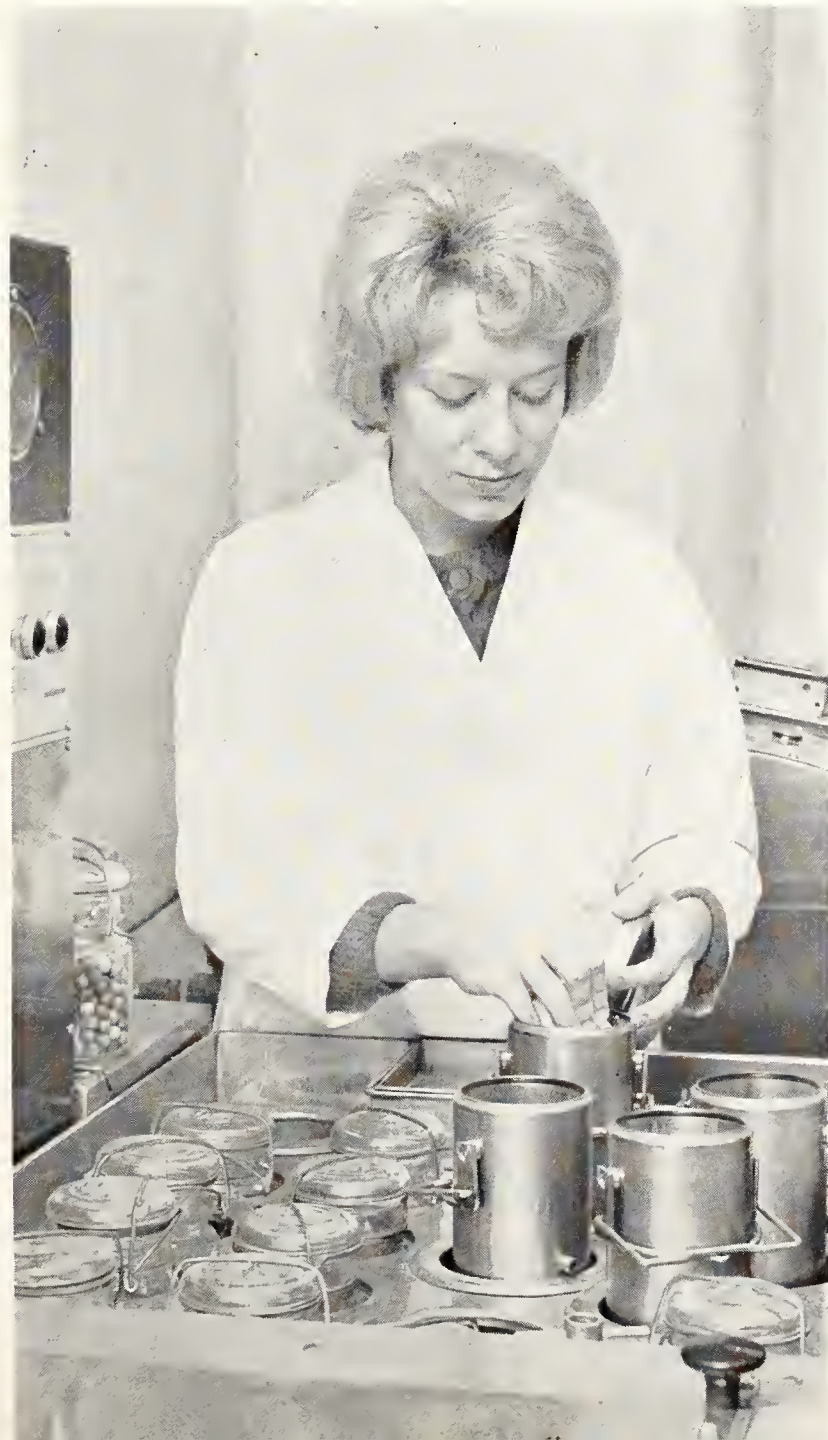
Textiles research utilizes the Launder-ometer to determine effects of soaps and detergents on fabrics.
