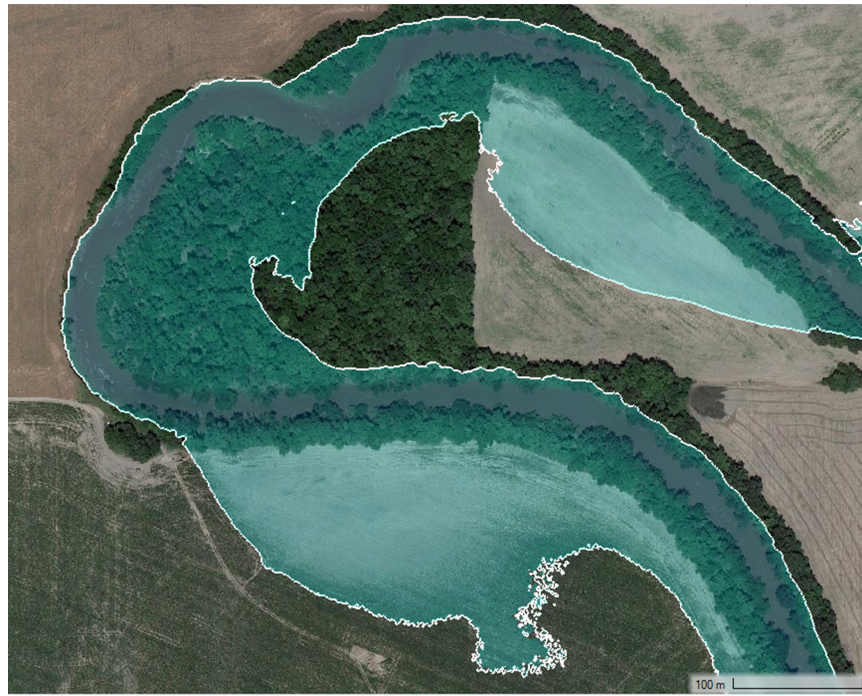
Figure 6.9: Example of 2D Hydraulic Model Calibration using June 27, 2019 Google Imagery showing May 2019 Flood Damage, Site 1.
