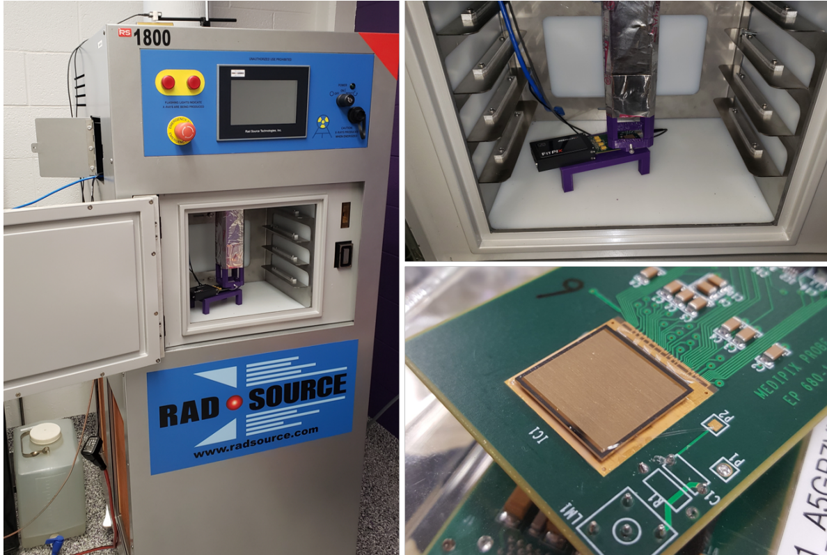
Figure 6.4: Left: Custom RS-1800 X-ray generator located in the Radiological Engineering Analysis Laboratory. Right: An X-MSND sensor card in-situ in the RS1800 and close up picture showing X-MSND/Timepix assembly. The card is aligned with the 3D printed x-ray occluder, directly in line with the RS1800 conical x-ray output.
