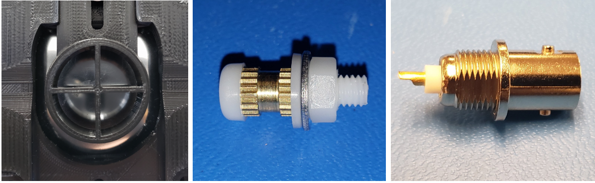
Figure 6.5: 3D printed PLA cross, xy oriented, 100% infilled. Cross has 1.5 mm thick arms with a 1 mm radius fillet on all junctions, 15 mm thick (right). Nylon M4 Phillips head screw with brass threaded insert, nylon washer, steel washer, and nylon nut (middle). Female BNC bulkhead feed-through; zinc and copper construction with Teflon insulator between conductors (right).
