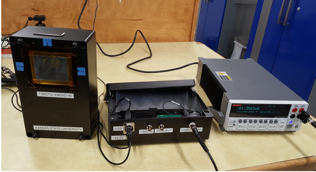
Figure 5.7: Light-tight probe card test boxes with Mylar window and feed-throughs. One test box is a redundant test vehicle. The sourcemeter for external negative bias is shown on the far right.
