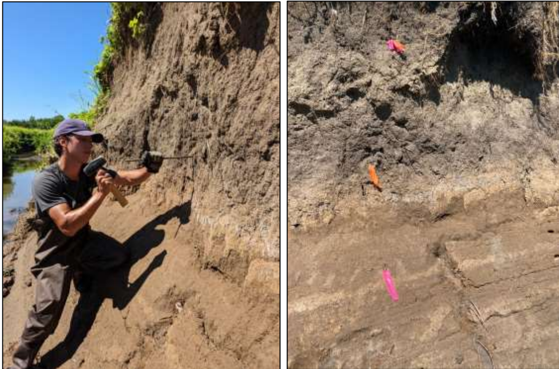
Figure 2.5 Rebar pins installed in the streambank revetment sites.
