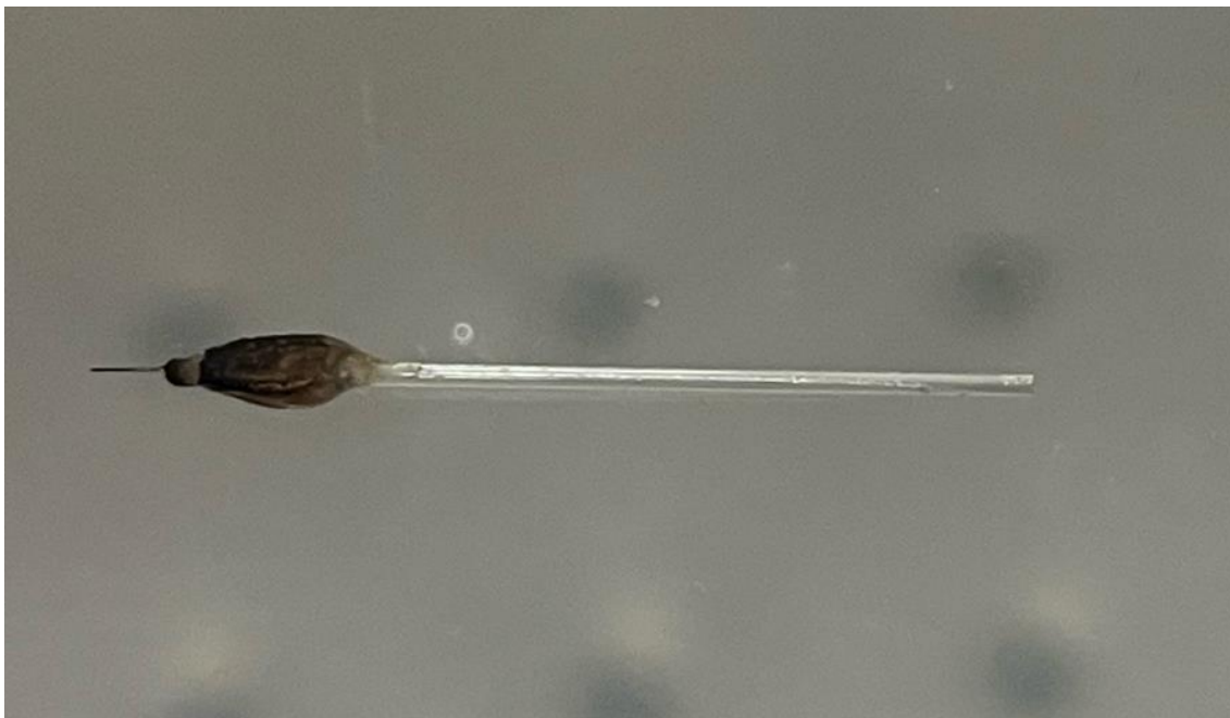
Figure 1. Melted capillary gauge-needle. This figure depicts the needle used in the injection experiments, which is a 34-gauge needle melted to the front of a capillary needle cut to six inches in length.
