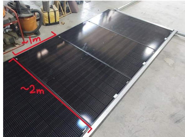
Figure 8 - Solar panels with markup showing approximate dimensions.
