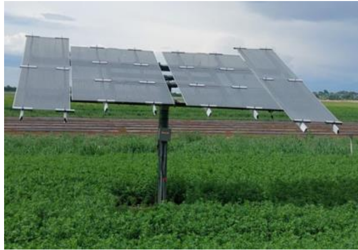
Figure 15 - Semi-Transparent panels over alfalfa crops outside Colorado State University's ARDEC Research Station
