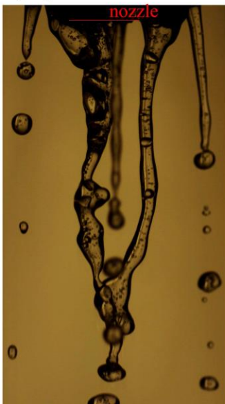
Figure 5.10 Spray from bubbler nozzles a) 6 psi bubbler nozzle distilled water spray with nozzle tip in view, b) 10 psi bubbler nozzle distilled water spray with top of image 2.0 mm from the tip of the nozzle, c) 15 psi bubbler nozzle distilled water spray with top of image 25.0 mm from tip of the nozzle, d) 6 psi bubbler nozzle surfactant solution spray with nozzle tip in view, e) 10 psi bubbler nozzle surfactant solution spray with top of image 46.0 mm from the tip of the nozzle, f) 15 psi bubbler nozzle surfactant solution spray 199.2 mm from the tip of the nozzle
