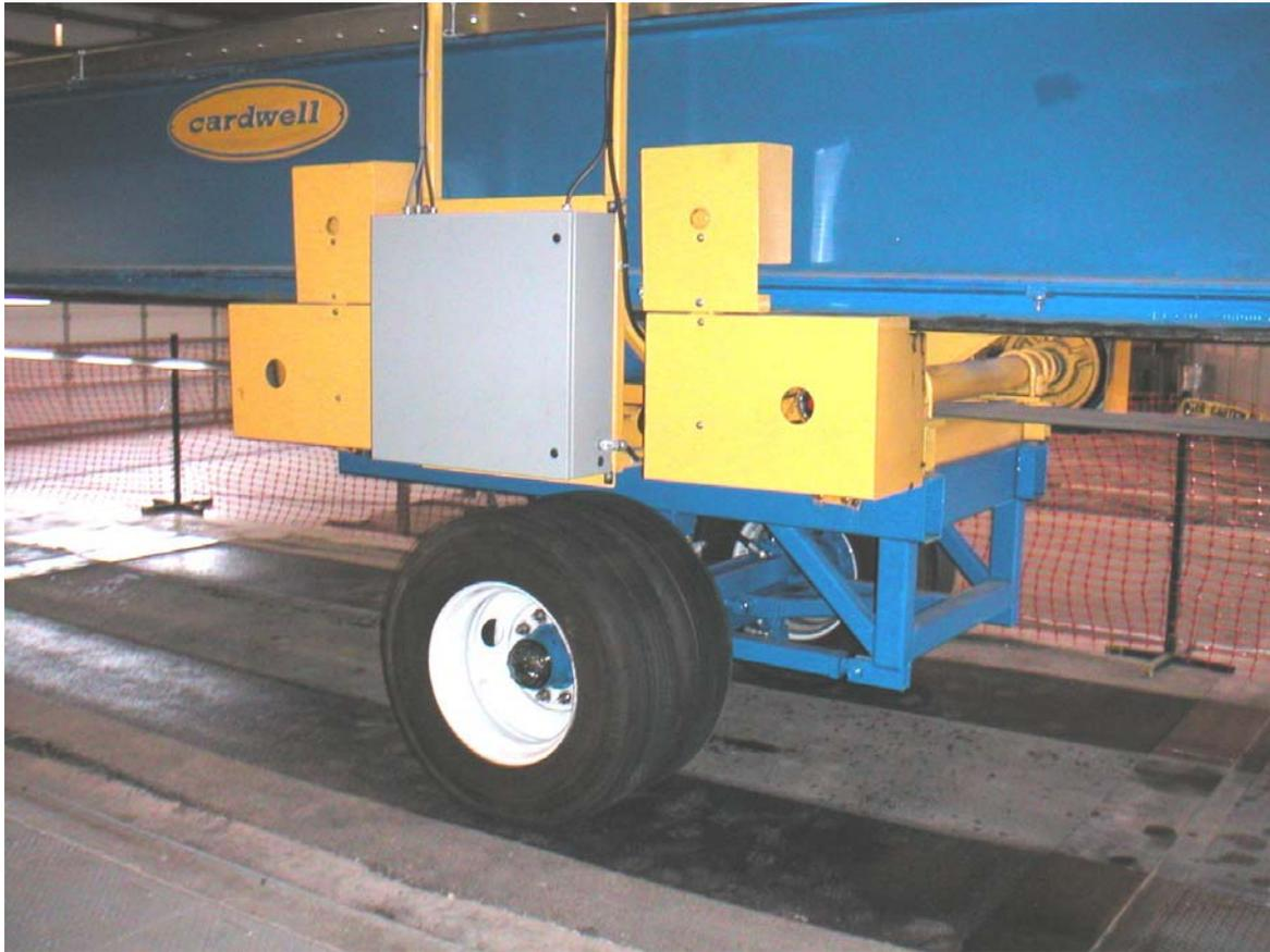
The machine is equipped with a lateral wandering device that moves the entire frame in a lateral direction with a maximum lateral wander of  $\pm 610$  mm ( $\pm 24$  inch). The lateral movement is applied in steps of 12.5 mm (0.5 inch). The lateral position of the frame (Figure 3.4) is controlled by an electronic controller (Figure 3.3). Provided in Table 3.1 are the number of wheel load passes at each lateral step.
