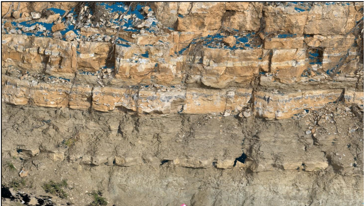
Figure 13. One point cloud, which are a product of >1000 photos per time sequence of the roadcut at Scenic Drive, visually indicating the kind of erosion that happened over a one-year timespan when compared with another point cloud of the same location. The blue color in the image shows NO DATA areas that Cloud Compare could not generate.
