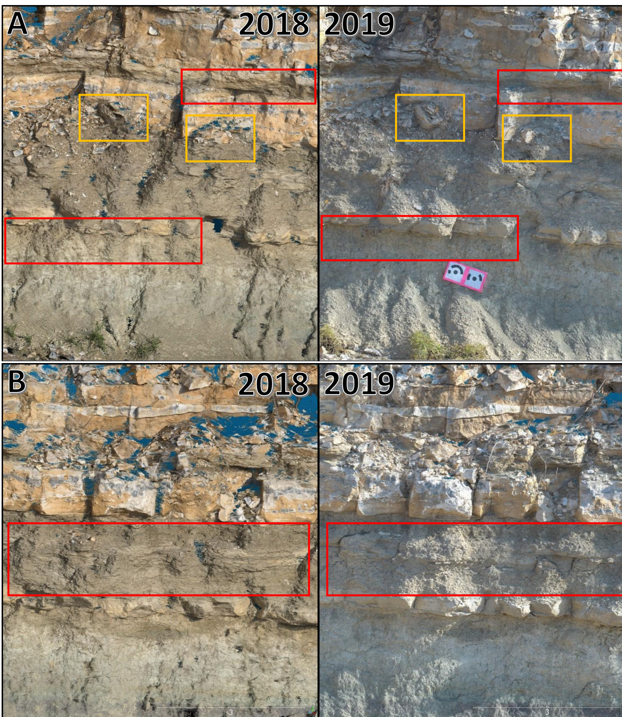
Figure 14. Comparisons of two point clouds, from November 2018 and 2019. Red boxes outline losses of shale. Golden boxes outline losses of limestone.
