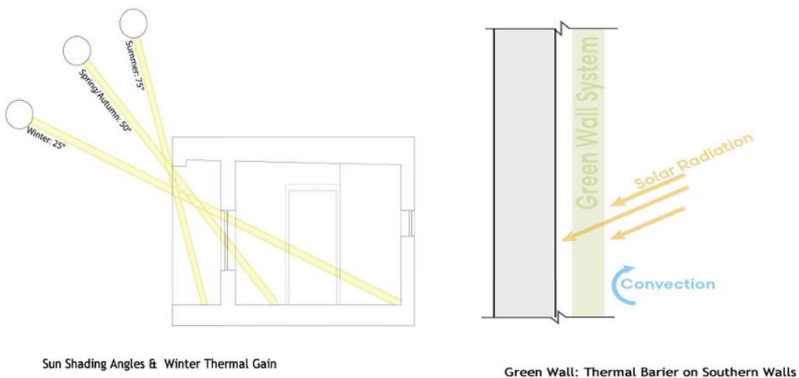
Figure 9. Sun Shading and Green Wall Diagrams
