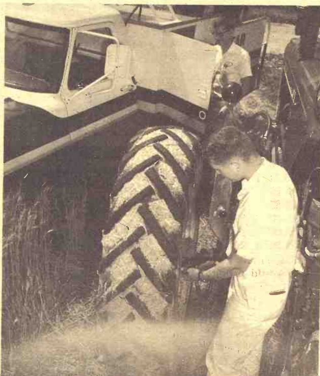
MAKING THE CHANGE. BRABEC AND ROSE PREPARE TO EXTRACT FLUID AND MOUNT NEW TIRES.
