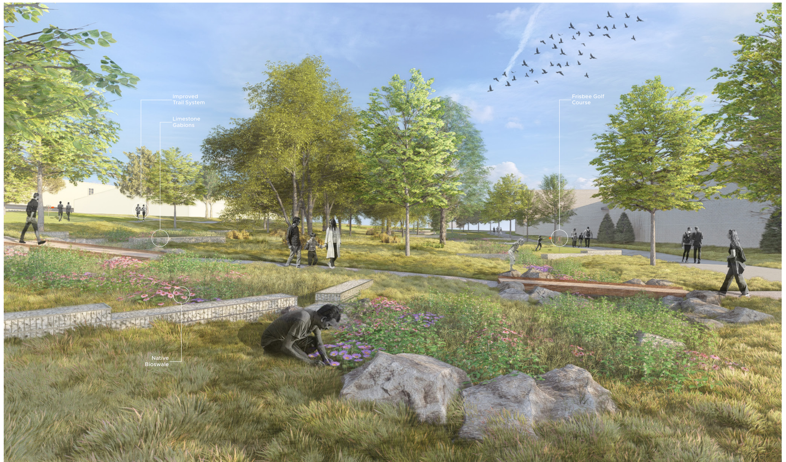
Fig 5.22 The enhanced swale allows for slower water movement, and a more aesthetic and functional landscape. (Freelove 2025).
