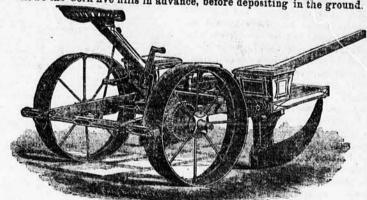
The Barlow Rotary, showing Drill Attachment attached.
