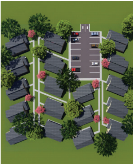
Figure 5.1 Illustrative plan view of housing type B in a Z-lot configuration
