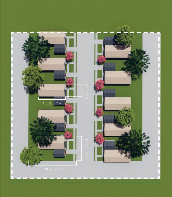
Figure 5.1 Illustrative plan of housing type A with zero lot lines NTS
