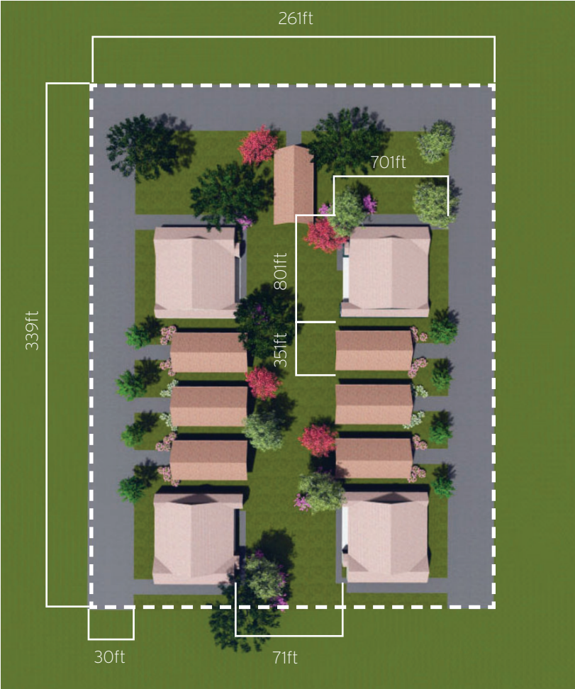
Figure 5.1 Illustrative plan view of a courtyard cluster with a medium wide courtyard
