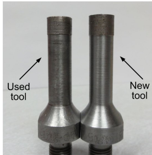
Figure 12.17 A new RUM tool and a used RUM tool after drilling more than 200 holes.
