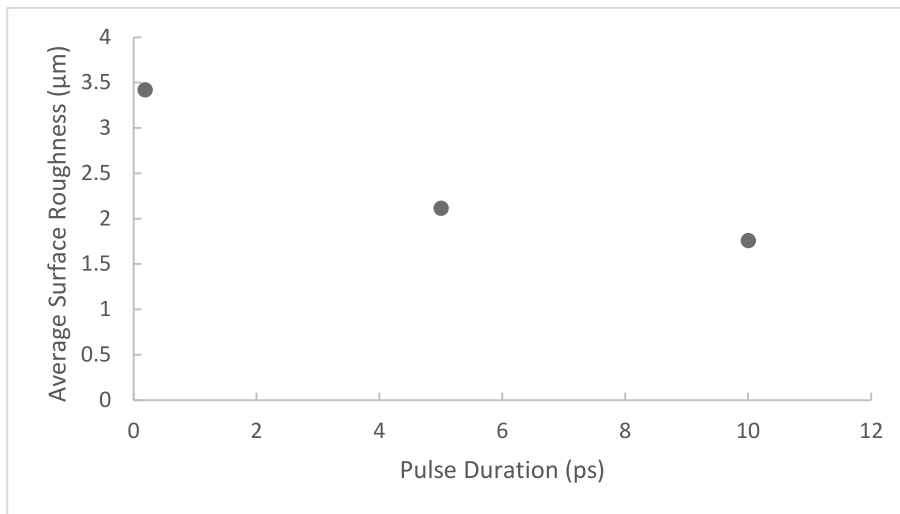
Figure 3.9 Effects of Pulse Duration on Average Surface Roughness
