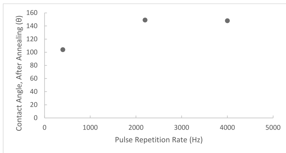
Figure 3.13 Effects of Pulse Repetition Rate on Contact Angle
