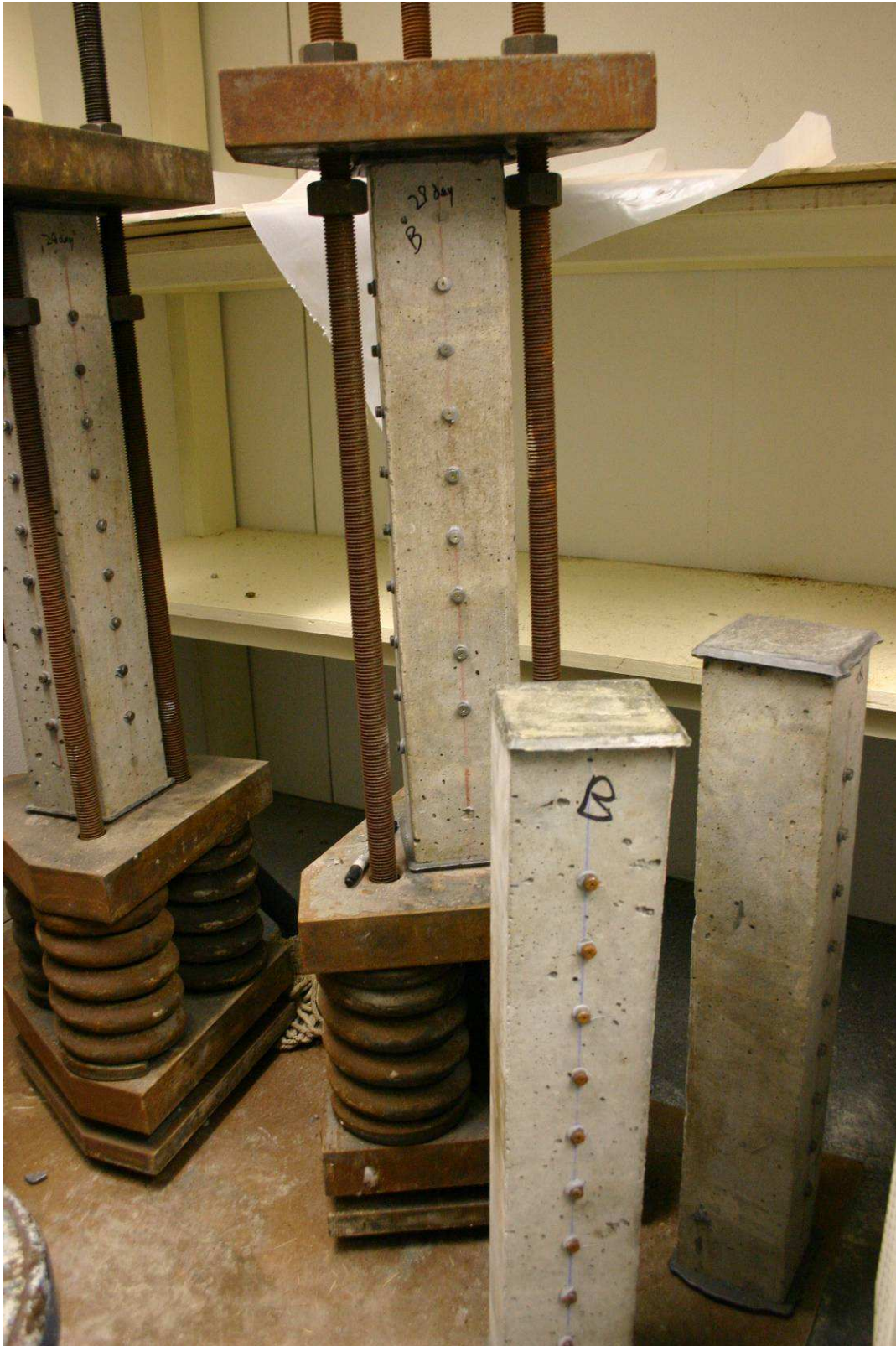
Figure 5.2 Creep prism in load frame
