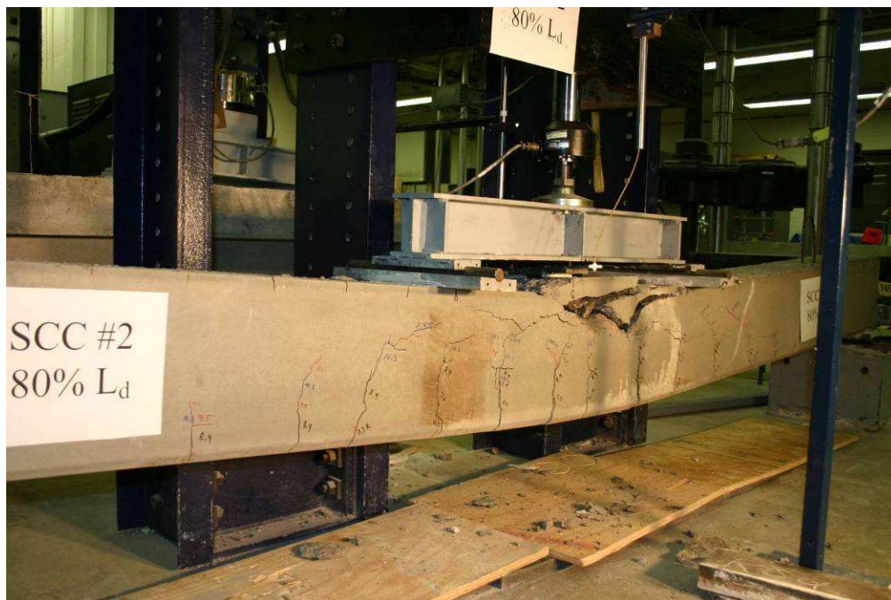
Figure 8.20 Failure of SCC #2 80% L d specimen
