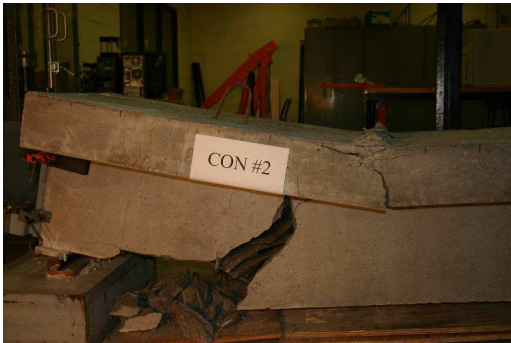
Figure 8.25 Failure of CON #2 T-beam specimen
