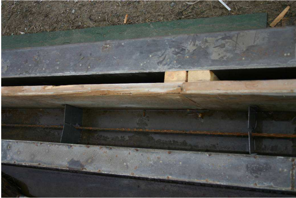
Figure 7.3 Crack formers in rectangular beams' form
