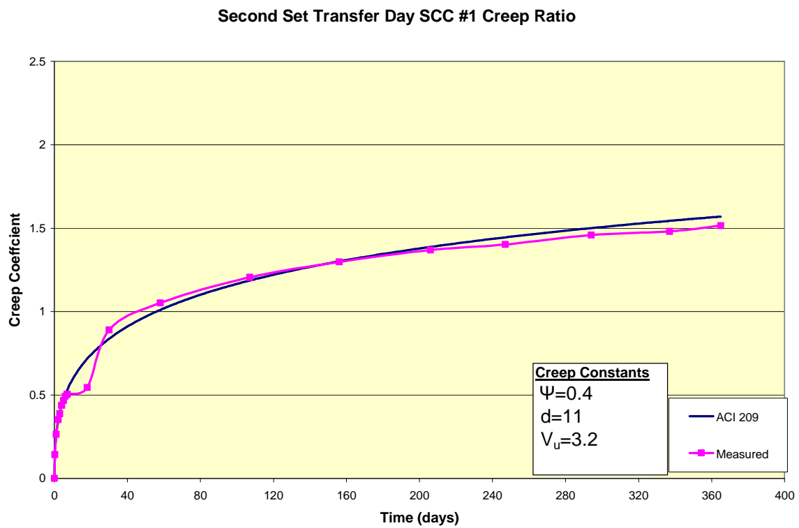
Figure 6.4 Creep coefficient of second set transfer day SCC #1
