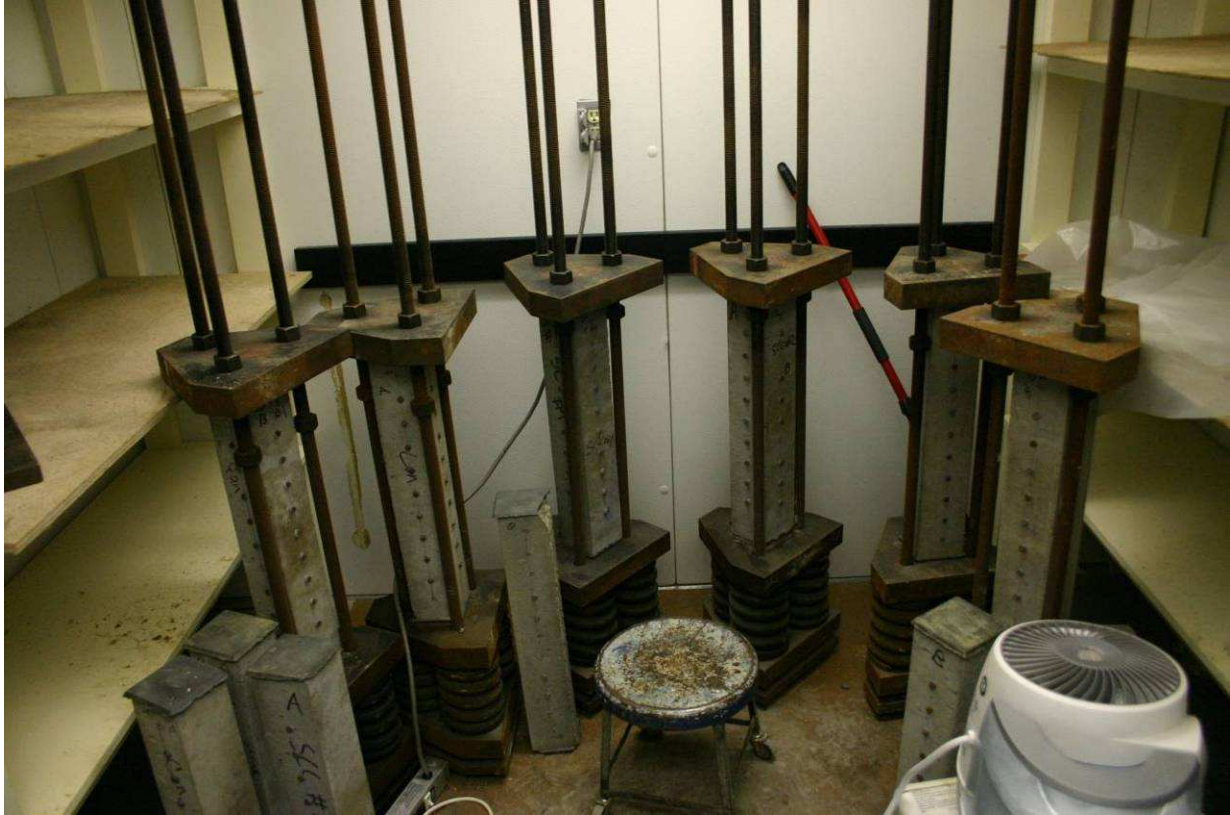
Figure 5.4 Second set of creep and shrinkage prisms in environmental chamber
