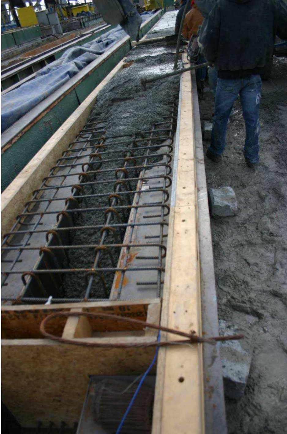
Figure 7.7 Casting of T-beam specimen
