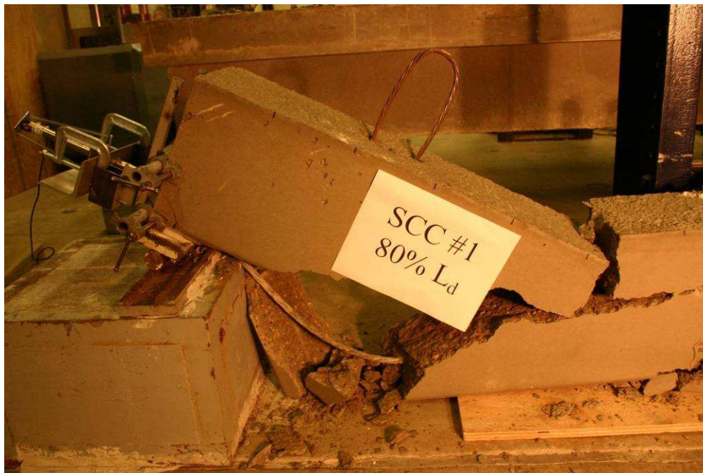
Figure 8.18 Failure of SCC #1 80% L d specimen
