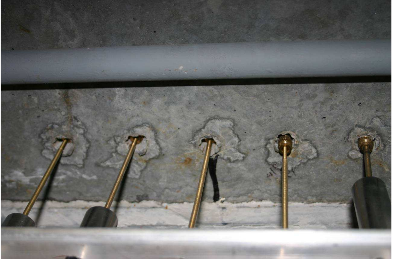
Figure 8.32 T-beam end after bond failure
