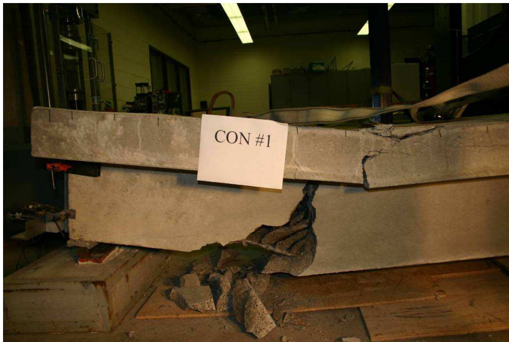
Figure 8.23 Failure of CON #1 T-beam specimen
