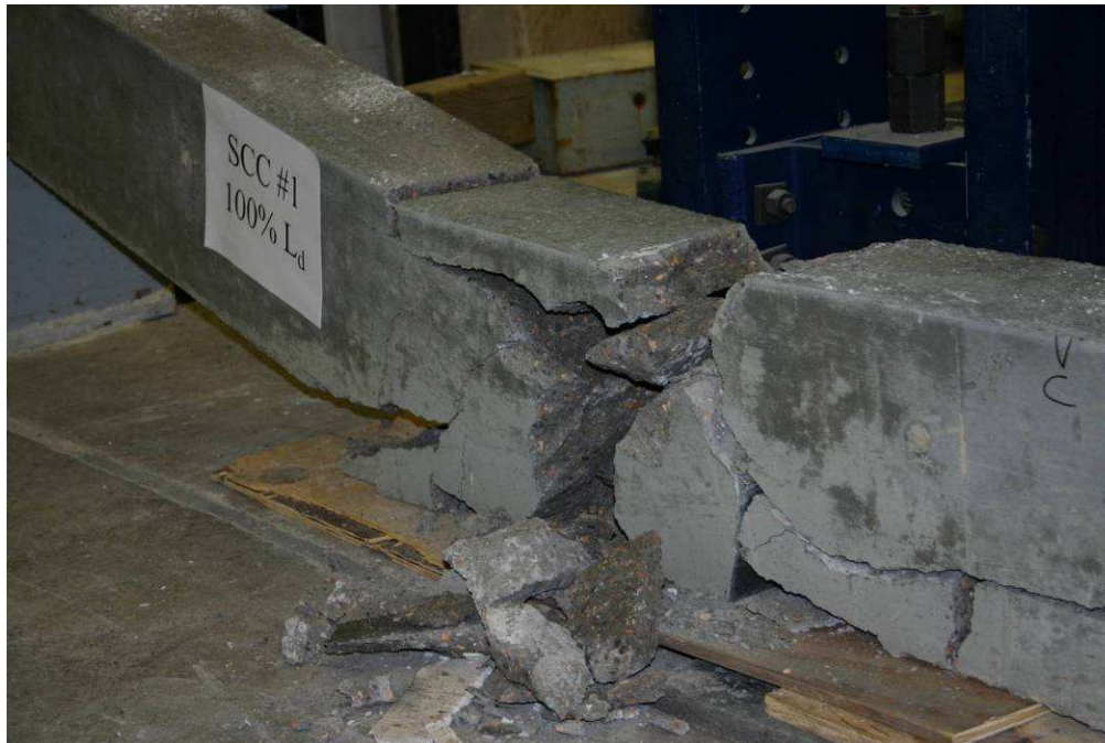
Figure 8.9 Failure of SCC #1 100% L d specimen
