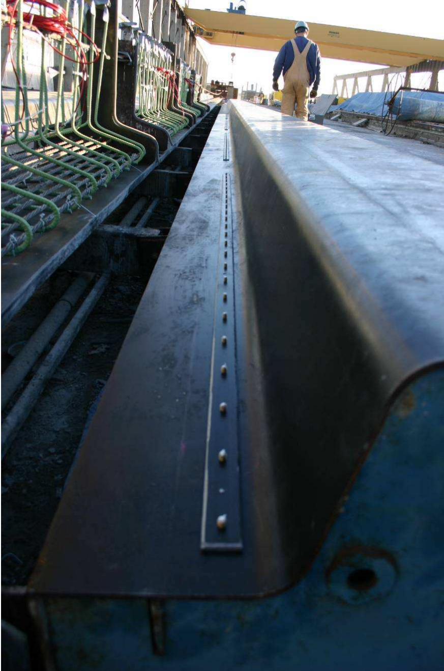
Figure 3.5 Whittemore points attached to IT forms
