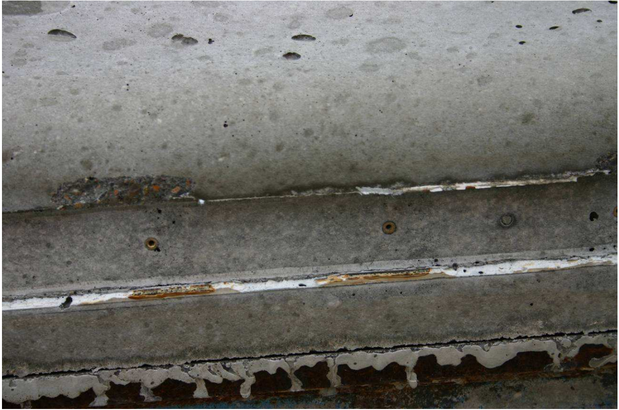
Figure 3.7 Whittemore points cast into ITs
