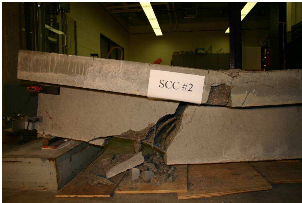
Figure 8.29 Failure of SCC #2 T-beam specimen
