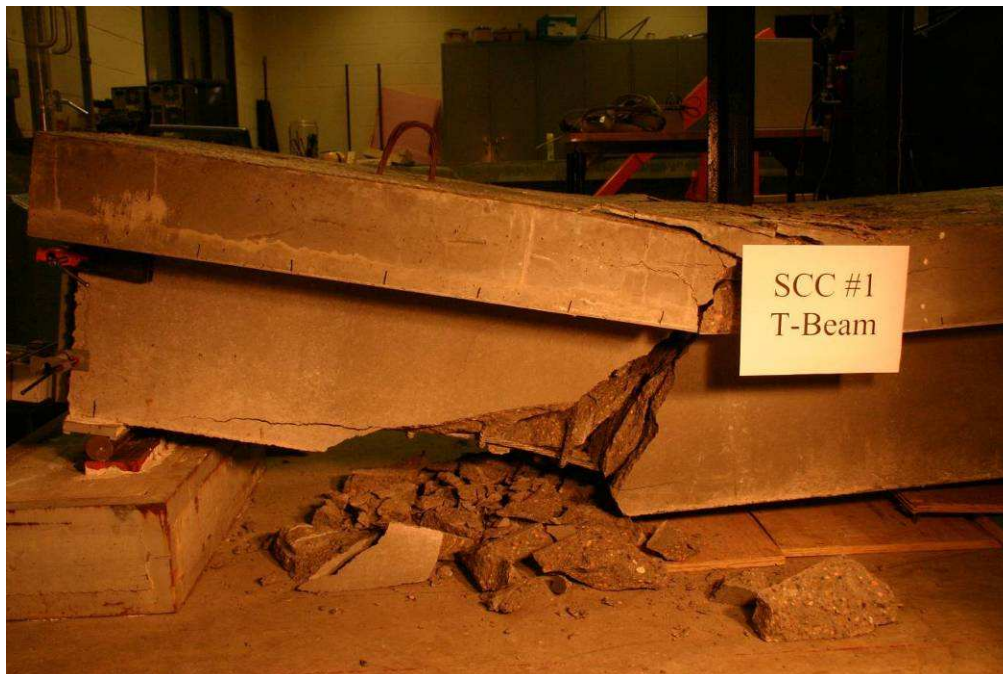
Figure 8.27 Failure of SCC #1 T-beam specimen
