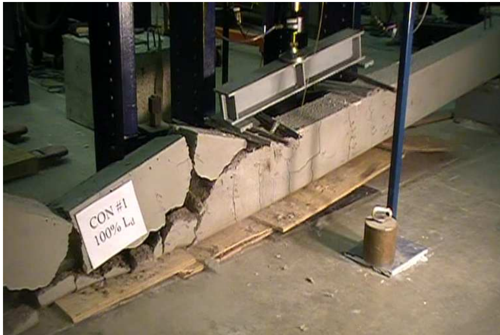
Figure 8.5 Failure of CON #1 100% L d specimen
