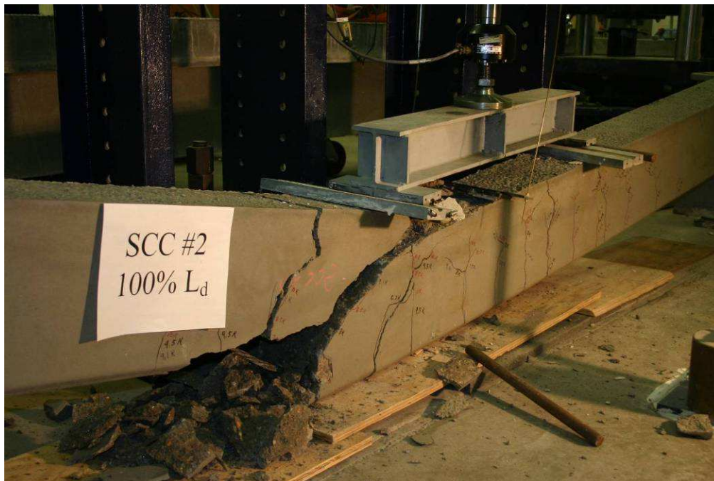
Figure 8.11 Failure of SCC #2 100% L d specimen
