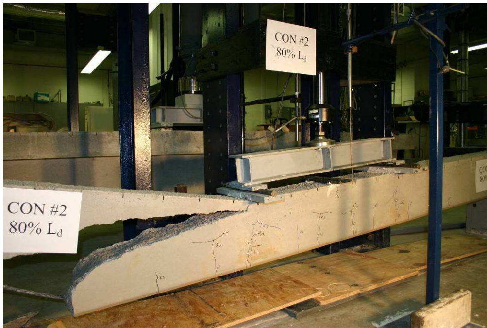
Figure 8.16 Failure of CON #2 80% L d specimen
