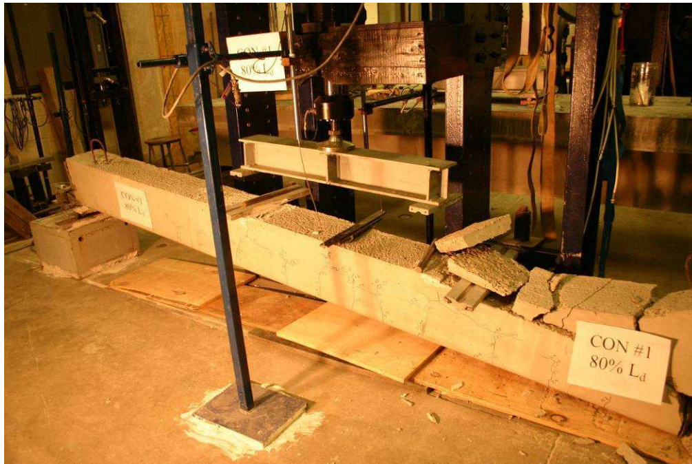
Figure 8.14 Failure of CON #1 80% L d specimen
