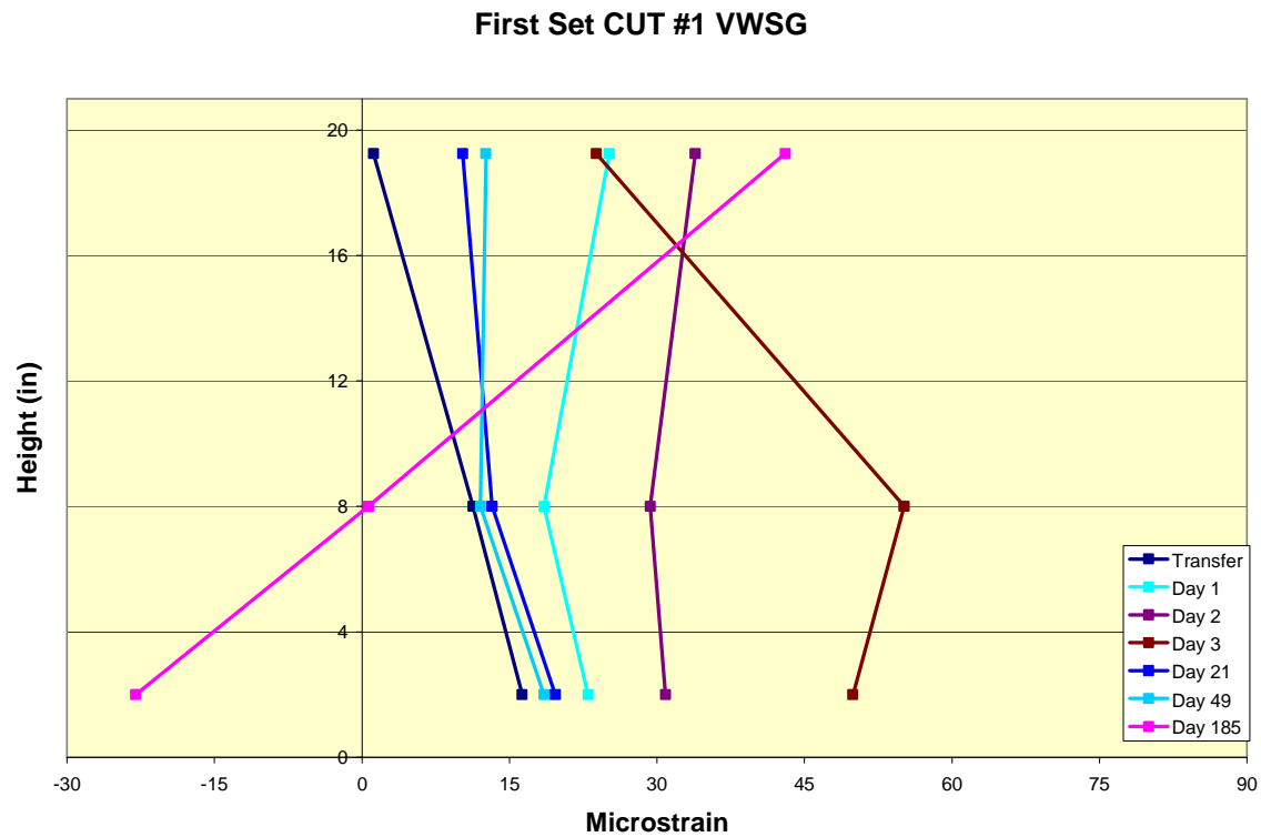
Figure 4.10 First set CUT #1 concrete strains (change due to shrinkage losses)
