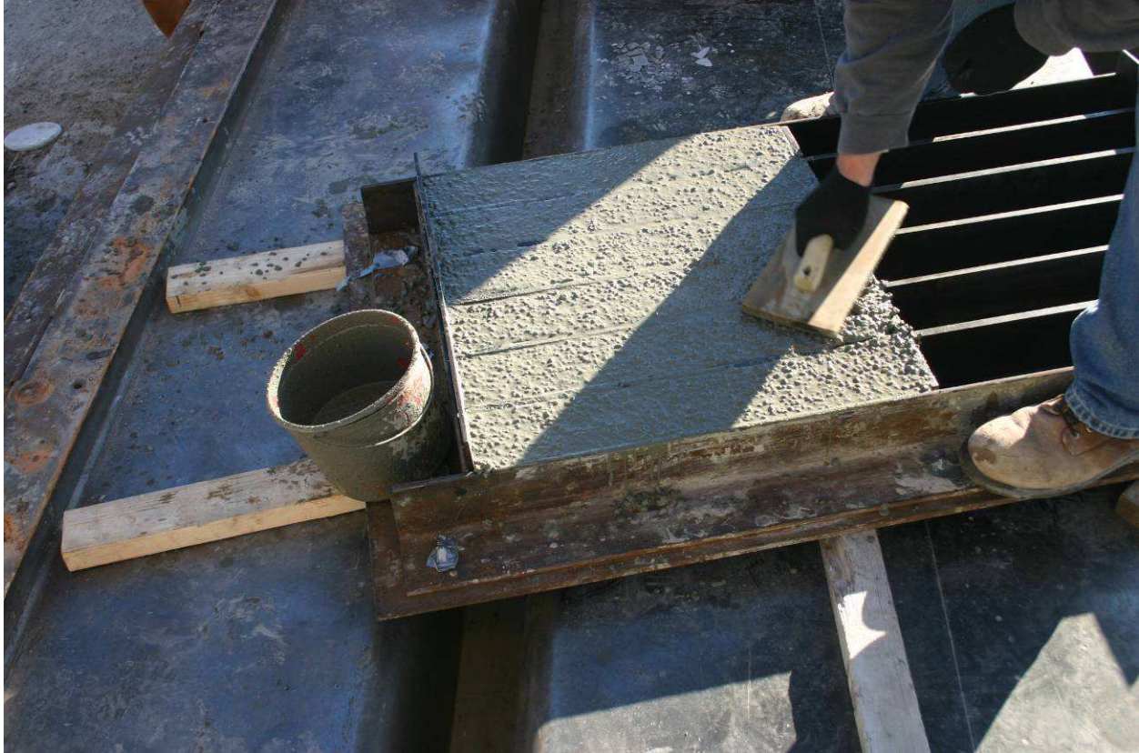
Figure 5.3 Casting of creep and shrinkage prisms
