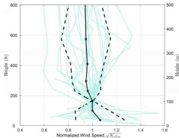
**Figure 3.2** Vertical profiles of normalized windspeeds for tornados (ASCE, 2021)
