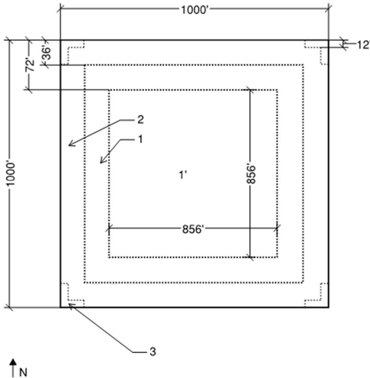
**Figure 4.2** Plan View of Power Plant with C&C Zones (NTS)
