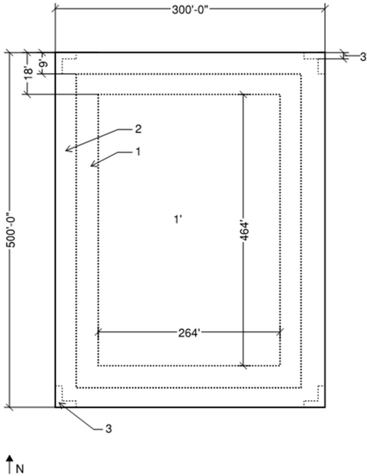
**Figure 4.1** Plan view of the elementary school with the C&C zones (NTS)
