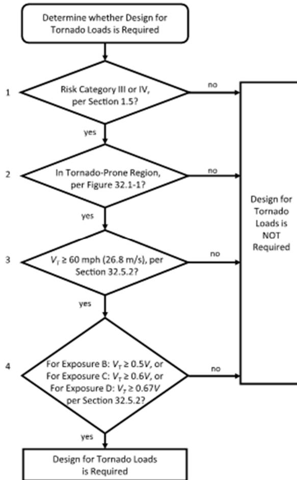
Figure 3.4 Flowchart for the process for determining when tornado loads are required. (ASCE, 2021)
