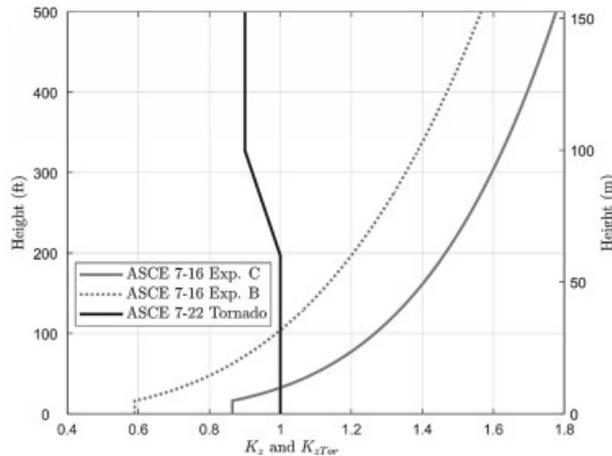
**Figure 3.3** Vertical profiles of tornado velocity pressure exposure coefficient ( $K_{zTor}$ ) (ASCE, 2021)
