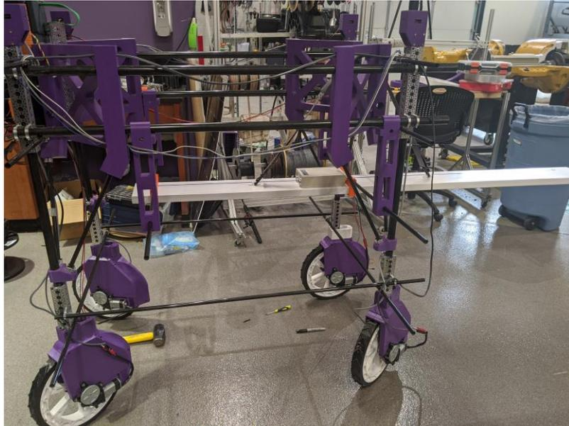
Additionally, as seen in Figure 2.25, there were carbon fiber crossbeams that were originally designed to be just above the fenders. With the addition of the gussets and the braces connecting to the wheel shaft, these lower cross braces would later be removed, reducing weight.
