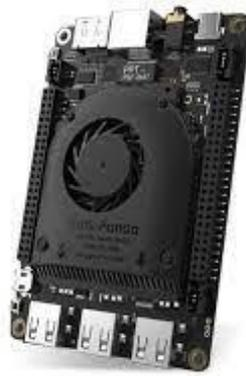
The LattePanda handles all the path planning of the robot. This is because the GPS is directly connected to the computer and the planned route is derived from planning the waypoints. In addition to the RTK GPS and waypoint path planning, the LattePanda also uses an object-detection program through Python TensorFlow.
