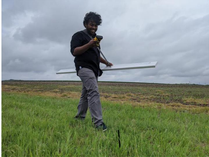
*Note.* Saquib walking the Geophex Sensor in the field to record test EM data
