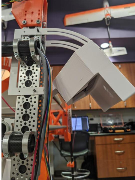
Figure 2.49 is a picture of the mounting system used to attach the camera to the robot. The camera is mounted close to the top of the shaft, nearest to the servos as possible. This allows the field of vision to be its largest while also maintain a fixed distance from the ground. The angle of the camera can then be adjusted from pointed straight at the ground to view the wheel to perpendicular to the ground, allowing the camera to observe more of the path ahead.
