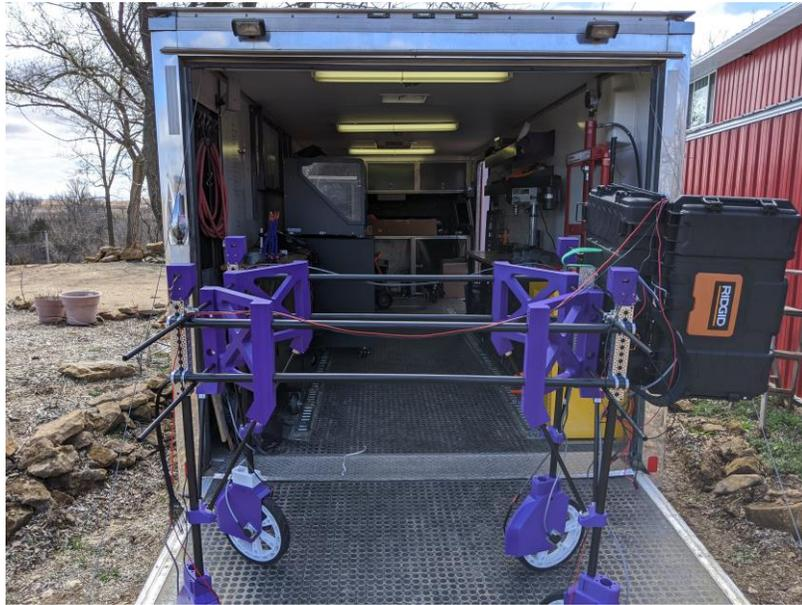
Figure 2.19 shows the designed gussets attached at the remote lab. Each corner of the robot has its own gusset that connects to the according wheel shaft. The result was greatly increased rigidity of the frame, as expected.
