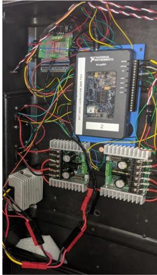
The servos are put into the 360-degree rotational setting, which can be adjusted via the button-layout configuration for the LSS HT smart servo. At the same time, the Sabertooth 32 A motor-controllers are set to be controlled via PWM directly from a battery powered microcontroller as specified by Sabertooth.
