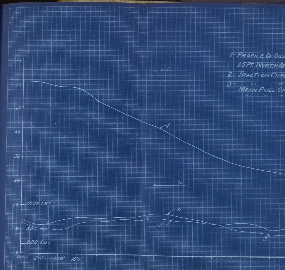
PLATE-1-1- PROFILE OF OILED ROAD FROM POINT 25FT. NORTHOF BRIDGE TO TOP OF HILL 2 - TRACTION CURVE ON ABOVE ROAD DRY WEATHER 3 - "" " " " " " " WET " WET
