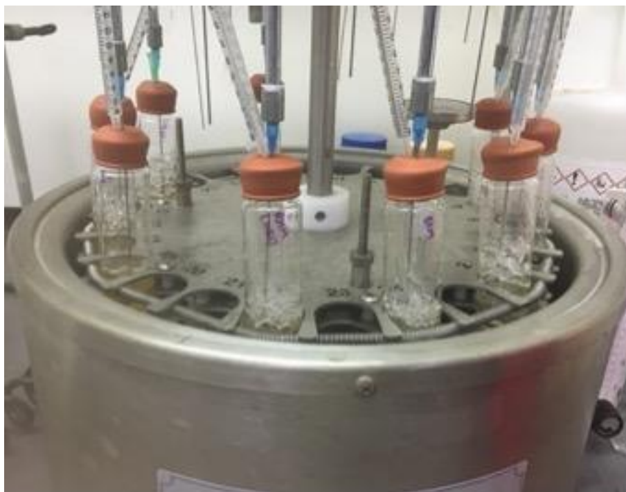
Appendix Figure A.4 Reactor setup for adsorption assay. Nitrogen gas was continuously blown into the tubes
