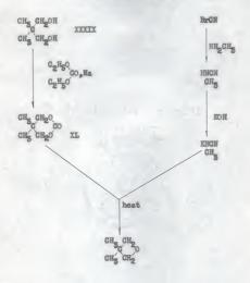
over potassium carbonate yields ethylene sulfide (38). Therefore, szetidines may be expected as a pyrolysis product of hexahydro-2-pyrimidones or tetra-hydro-1.3-oxszin-2-ones over an alkali catalyst.
