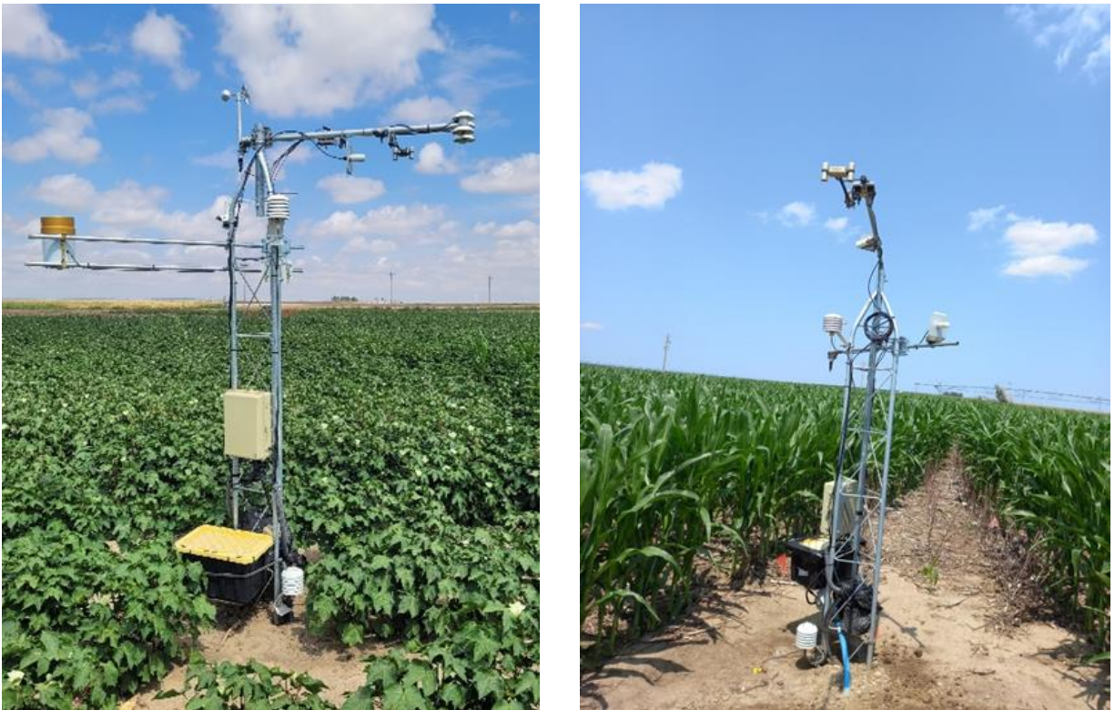
Figure 3.4: Instrumentational setup of energy budget towers in cotton (left image) and corn fields (right image).
