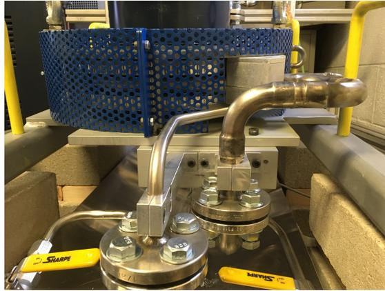
Figure A.2: Suction (inlet) flanges of the GaTE pump.
