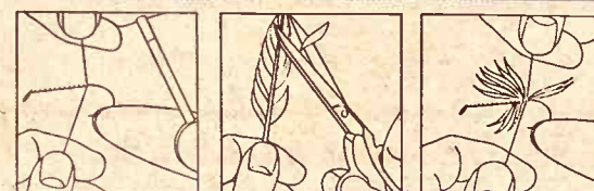
1. Clamp hook in fly-tying vise, wrap with thread. 2. Cut wings, tail from feather. Attach to hook. 3. Shape feathers to resemble bug.
