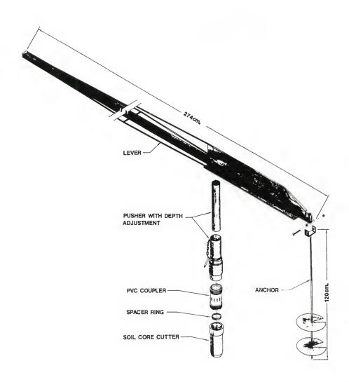
Figure 1. Undisturbed soil core sampling apparatus.
