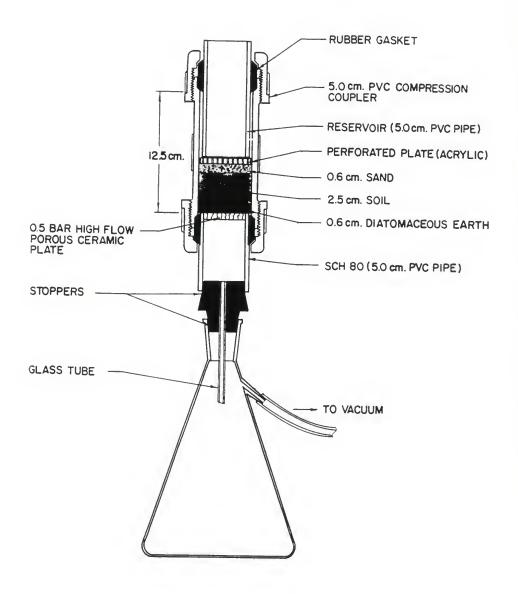
Figure 2. Undisturbed soil core leaching apparatus.
