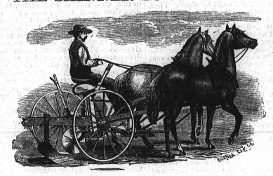
Can furnish either right or left hand Sulky Plows, old ground or prairie breaker irons. It can be changed from one to the other in five minutes, by merely substituting different plow irons.
