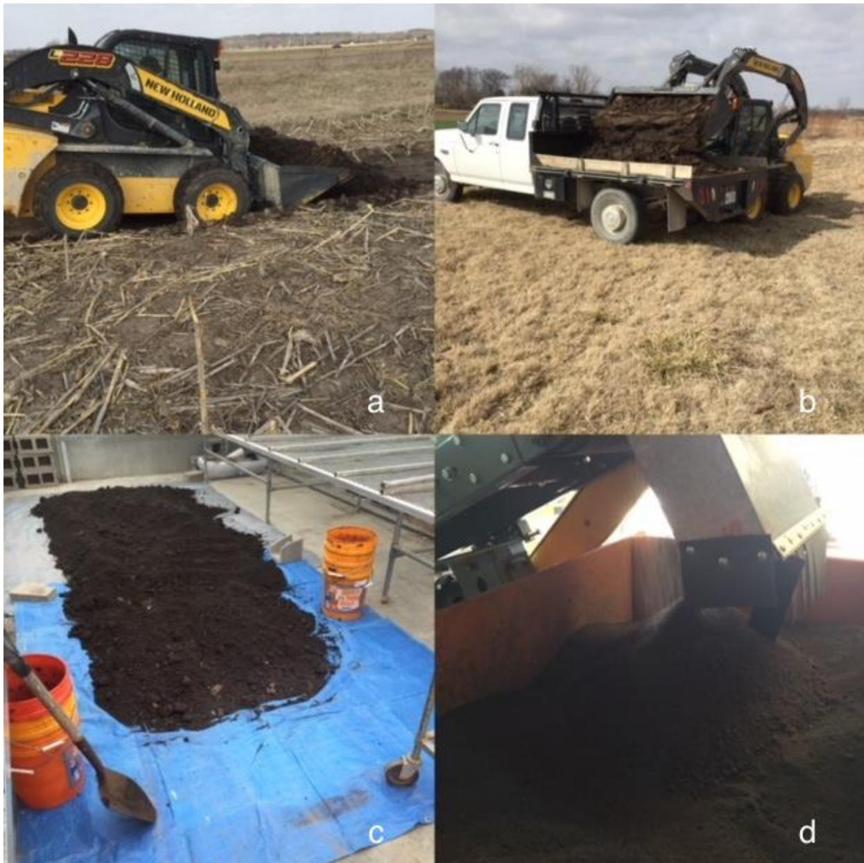
**Figure 3.14** Preparation of soil mixture (a. removal of top residue, b. collection of soil, c. laying soil out to dry, d. mixing soil with washed sand (1:2 ratio).)
