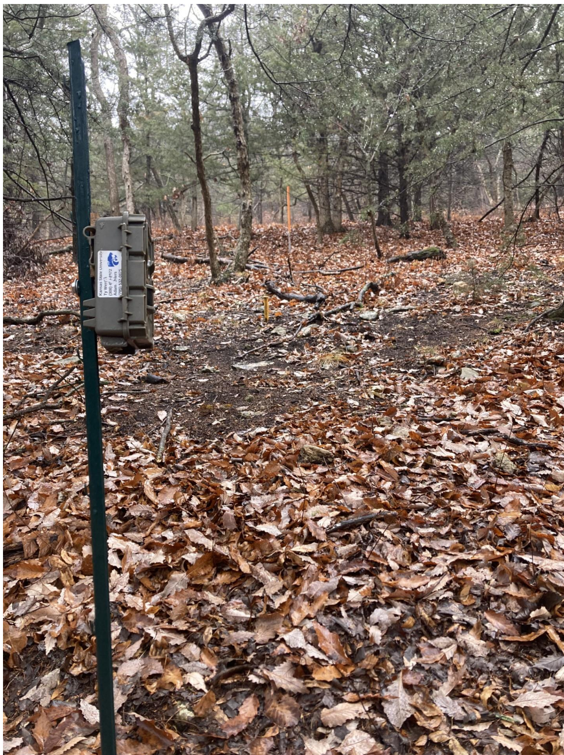
Appendix Figure B.2. Camera setup 0.5 meters off the ground in a Burn Only area near a preexisting t-post.
