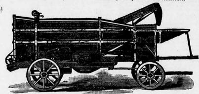
Giant and Stillwater Traction Farm Engines FRICTION CLUTCH, RETURN FLUES, BURN WOOD, COAL OR STRAW.
