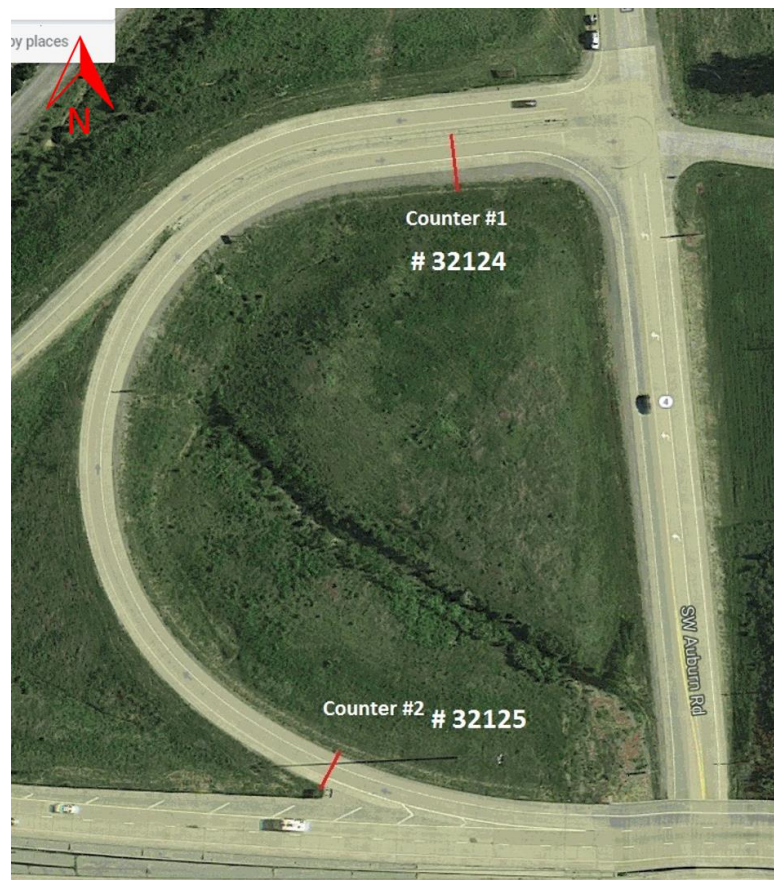
Figure 5.10: Road Tube Layout Used for Data Collection (Google 2020)
