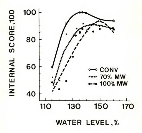
Effect of water level on the quality of cakes baked by conventional means -  $\sf Estimates$  , and  $\sf R^2$  and  $\sf F$  values from analysis of variance of forward multiple regression solution Table 9.
