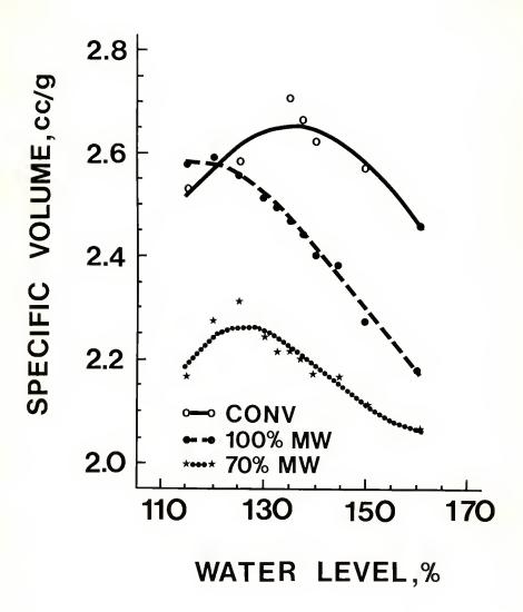
Figure 3. Effect of water level on crumb compression for cakes baked by conventional means and with microwave energy at 70% and 100% power levels.
