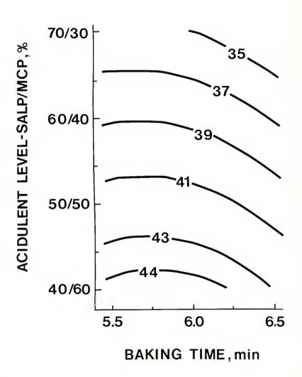
Figure 14. Contour plot of crumb pH for different baking times and acidulent levels for cakes baked with microwave energy.
