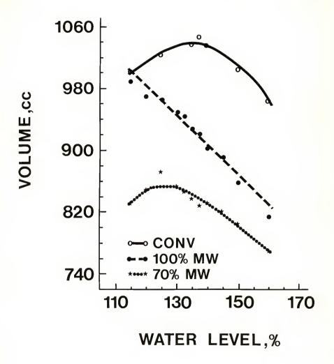
Figure 2. Effect of water level on specific volume for cakes baked by conventional means and with microwave energy at 70% and 100% power levels.
