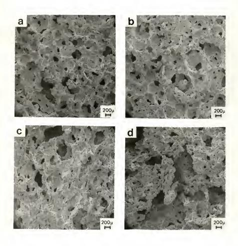
For both positions in the conventional cake, increased baking time did not appear to affect the cell structure.
