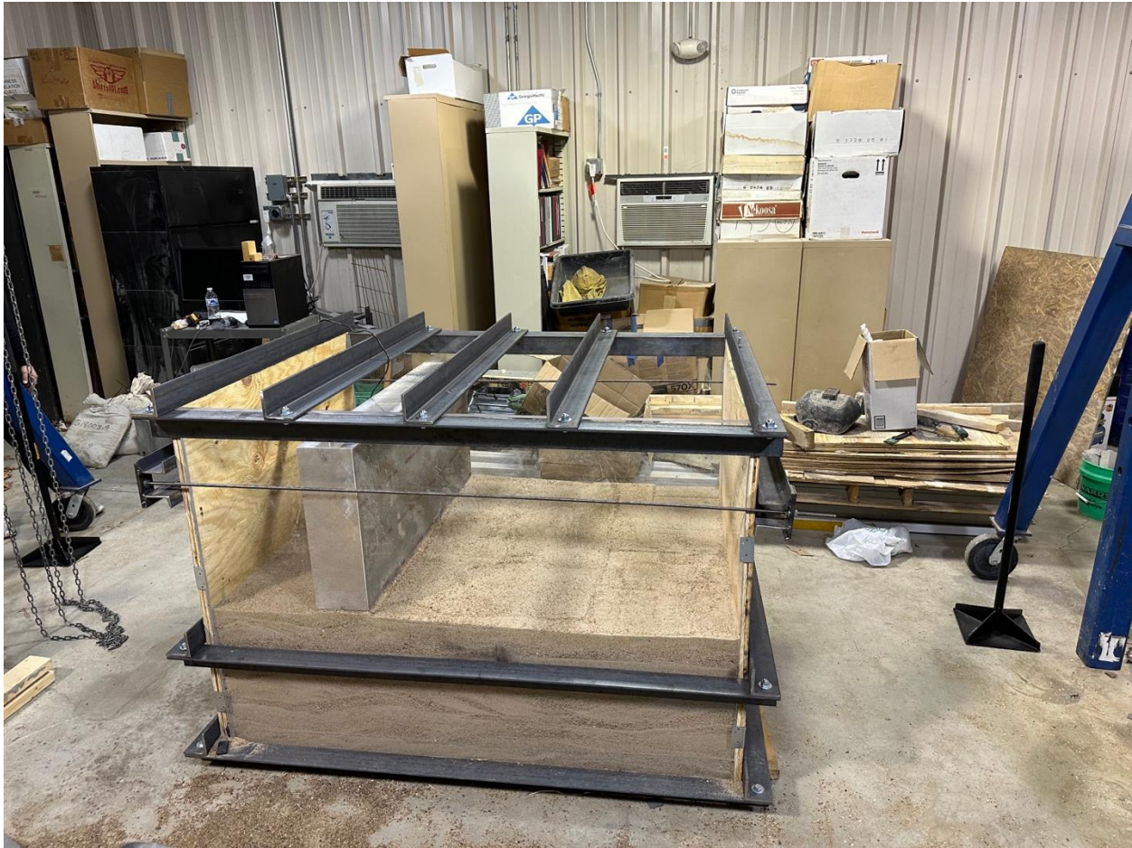
Figure 3-3 View of Steel Angles Used for Bracing
