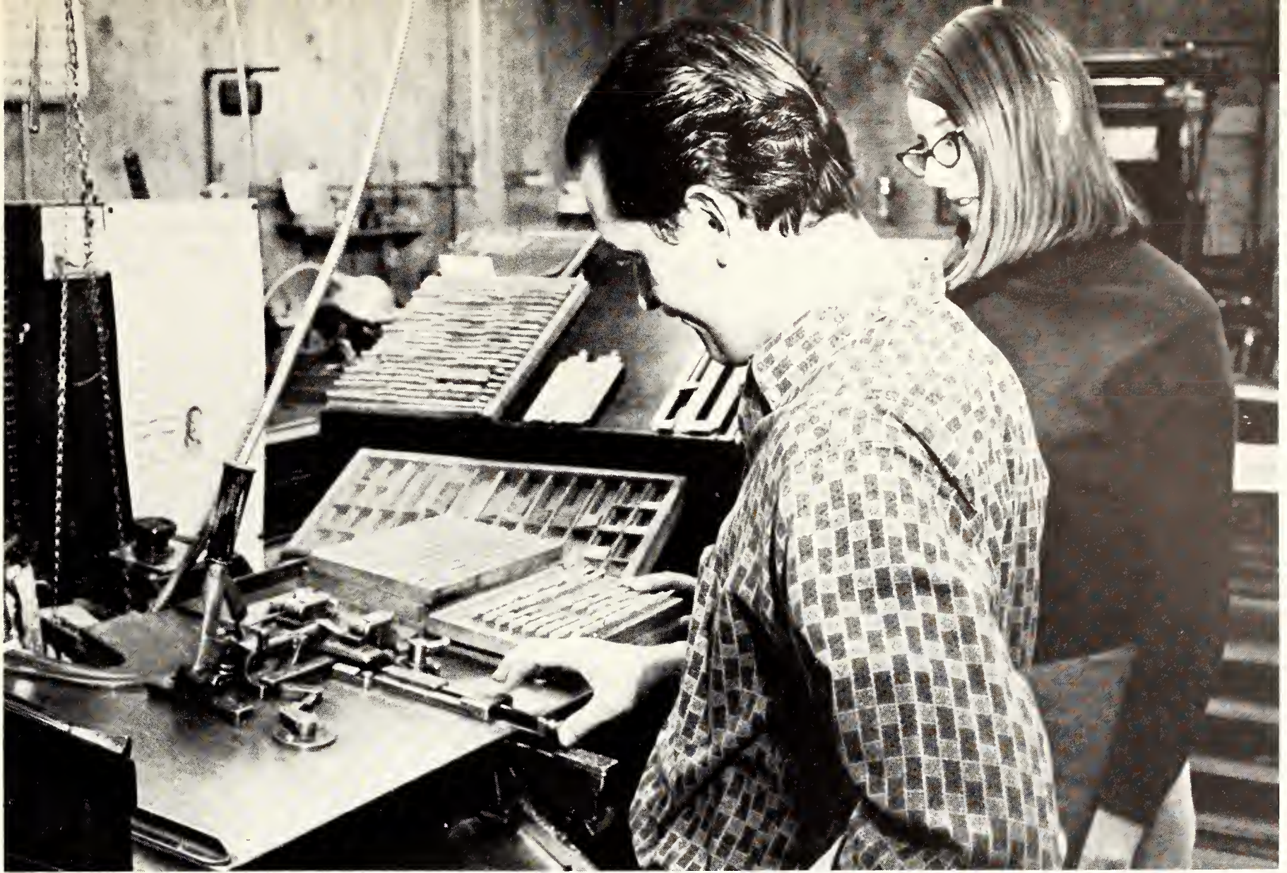
Collegian editors check a headline for length after it is set in hot lead on a Ludlow machine. Each morning before the paper
